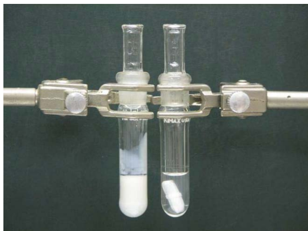
Fig. 4 Right: \text{Na}^+ -complex 2 in \text{CHCl}_3 after the extraction. Left: same solution after bubbling \text{CO}_2 .
